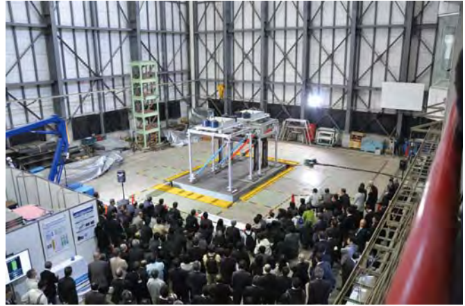
Vibration testing of a buckling-restrained brace
