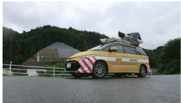
Measuring the cut slope of a construction site with MMS
