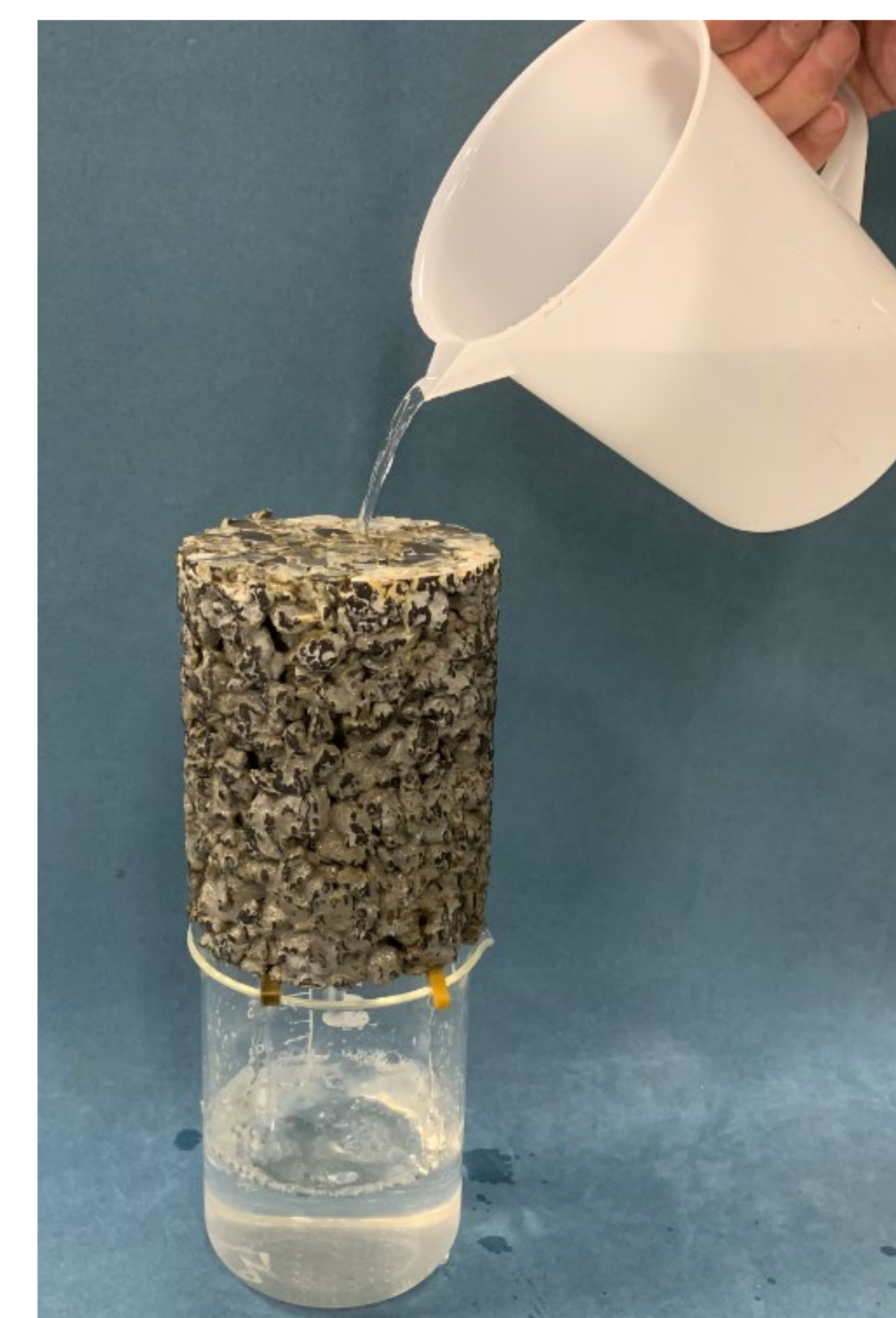
Permeable improvement body Hydraulic conductivity k=1.0 \times 10^{-3} \text{m/sec}
