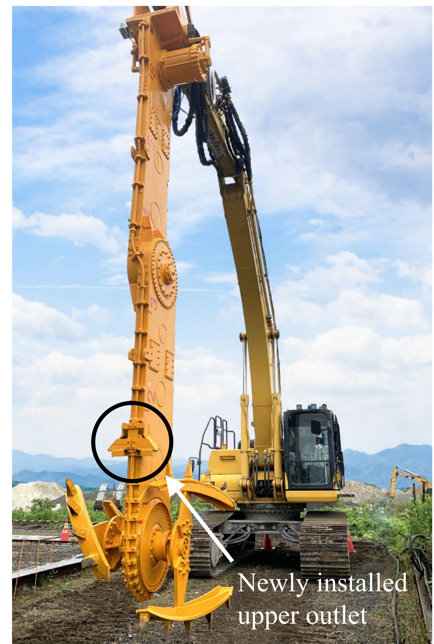
Construction machine of WILL-m method
